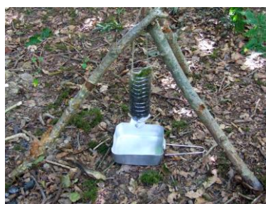
An improvised water filter
