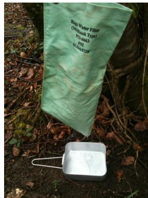
The Milbank bag set up with mess tin to collect the filtered water
