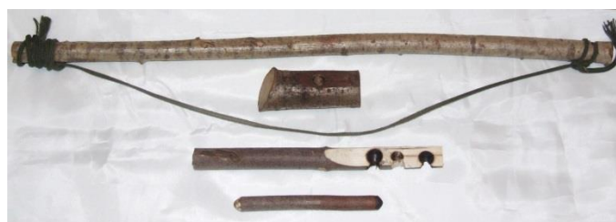
A sycamore drill and base board with a bow and hand block
